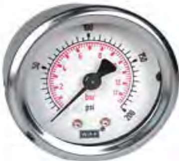
A380653-2 Air Pressure, 0-200psi 1/4"MNPT Back Mount
